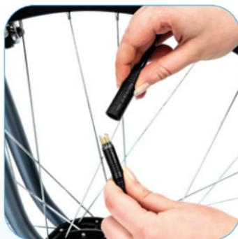
8. Combine the cable coming out of the bracket with the cable coming out of the motor, while doing this, make sure that the arrows on the cables point to each other. Fix the cables without restricting the mobility of your handlebar with the clips included in the package.
