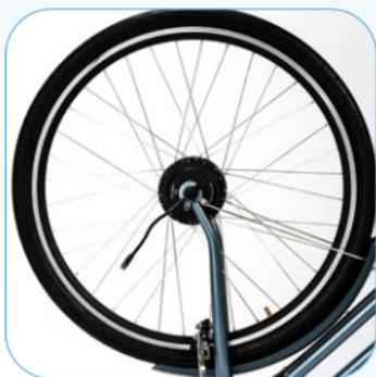
3. Put your ordinary rim aside and attach your tire to the e-motorized front rim (with the help of the tire lever or the back of the spoon) from the Byqee box.
