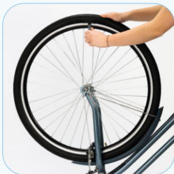
2. Remove the nuts on the front fork. Remove the ordinary front wheel, deflate the tire, then separate the tire from the rim (with the help of the tire lever or spoon handle). If you wish, you can do this by turning the bike upside down.
