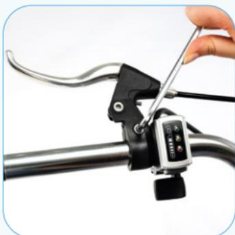
7. Attach the throttle as you are comfortable and fix it with the help of the allen key.
