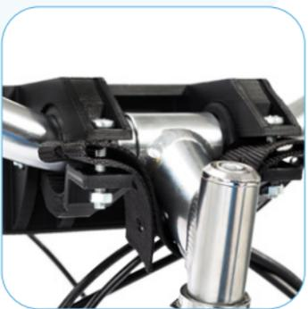
5. Place the bracket in the middle of the handlebar. Thread the belt that comes out of the Byqee package into the bracket's tabs so that it passes under the bike stem. Fix the bracket to the handlebar with the screws included in the package. Note: Make sure the rubbers and belt are installed correctly.
