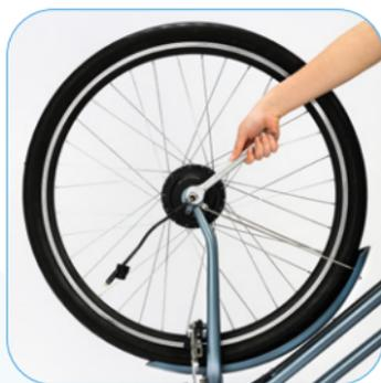
4. Inflate your tire and place your tire. Install the motor nuts and tighten them with the wrench. Install the brake cable and check the other brake assemblies if any and be sure to start. The motor cable should remain on the right for 100mm motors and on the left for 74mm motors.
