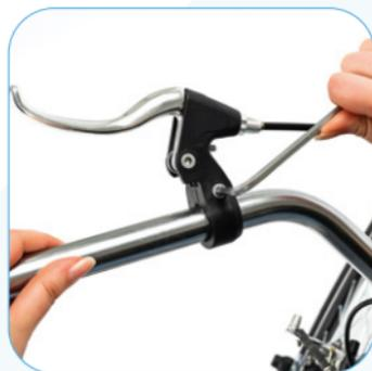
6. Remove the grip on the side where you will attach the throttle lever of the handlebar (you can easily do this by squeezing cologne into the grip). Remove the brake lever (optional).
